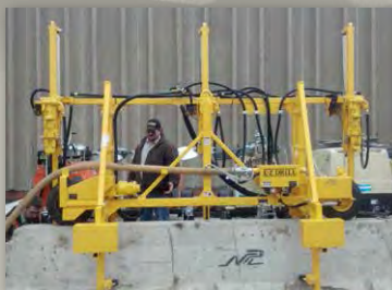
3-GANG PARAPET WALL DRILL
